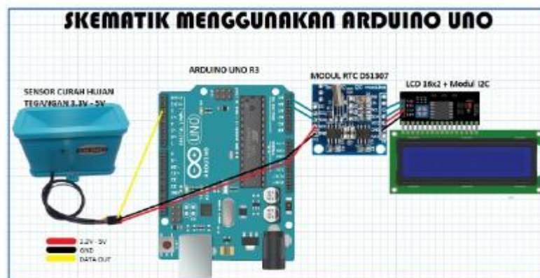
Figure 5: Arduino schematic circuit
